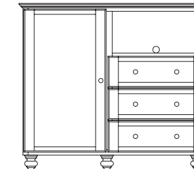
micro/fridge chest left 54.25" w x 24.125" d x 48" h microwave opening: 21" w x 20.75" d x 12" h refrigerator opening: 21" w x 20.75" d x 33.75" h 3 drawers with ball bearing glides recessed / vented back 1 fixed shelf high pressure laminate top with solid wood beveled edge
