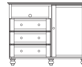
media chest right 54.25" w x 24.125" d x 42" h media opening: 25" w x 20.75" d x 7.5" h 3 drawers with ball bearing glides recessed / vented back 1 fixed shelf high pressure laminate top with solid wood beveled edge
