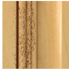
#10 - WORMHOLING (ADD 10%) Closely grouped holes with beaten grain.
